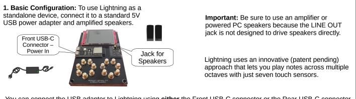
You can connect the USB adapter to Lightning using **either** the Front USB-C connector or the Rear USB-C connector on the left side of the device. We recommend the Front USB-C because the Back USB-C is generally for USB data.
