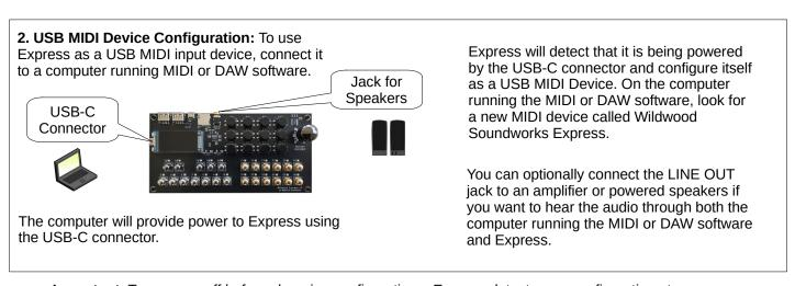
Important: Turn power off before changing configuration – Express detects new configuration at power-on
